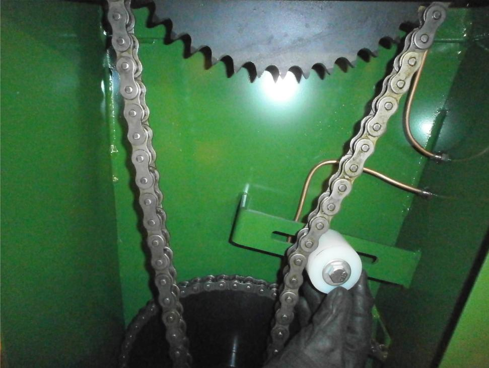
5) Make sure the front spider gear is contacting the reel drive.
