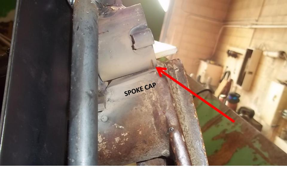
Put the paddle assembly on the spoke and see if the paddles touch here. If they do then grind a little off the spoke cap unit the paddle moves freely.
